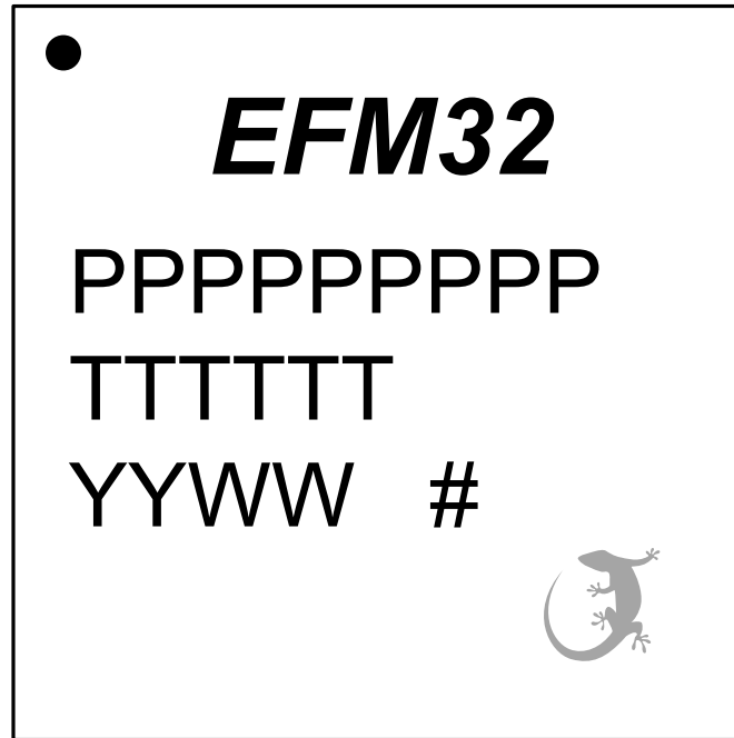
Figure 7.3. QFN48 Package Marking
