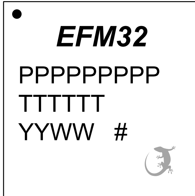
Figure 7.3. QFN48 Package Marking
