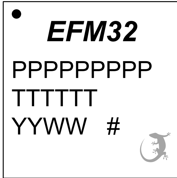
Figure 8.3. QFN32 Package Marking
