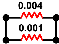
FIGURE 117. A SIMPLIFIED SCHEMATIC ILLUSTRATING THE USE OF TWO SHUNT RESISTORS TO CREATE A DESIRED SHUNT VALUE
