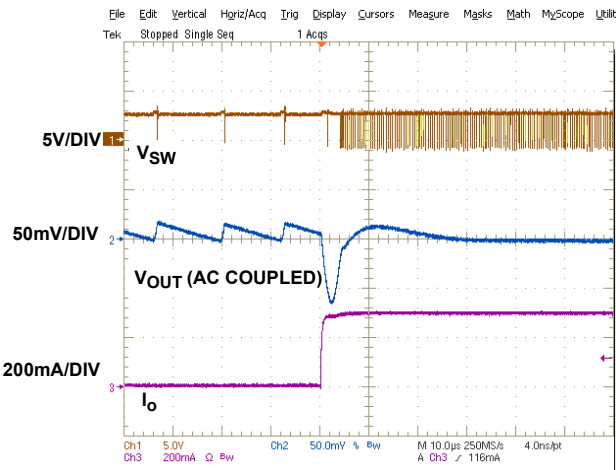
FIGURE 17. LOAD TRANSIENT FROM PFM TO PWM MODE ( V_{IN} = 3.6V , V_{OUT} = 2.5V , 5mA TO 300mA)
