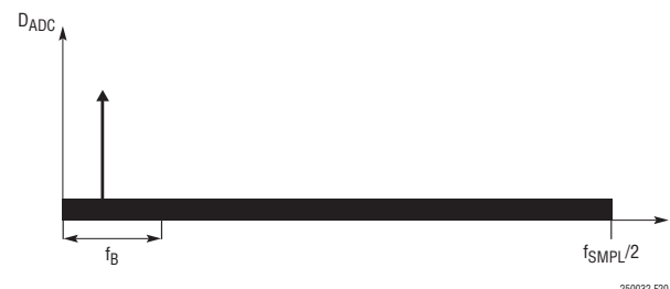
Figure 20. Frequency Spectrum of SAR ADC Core Output
