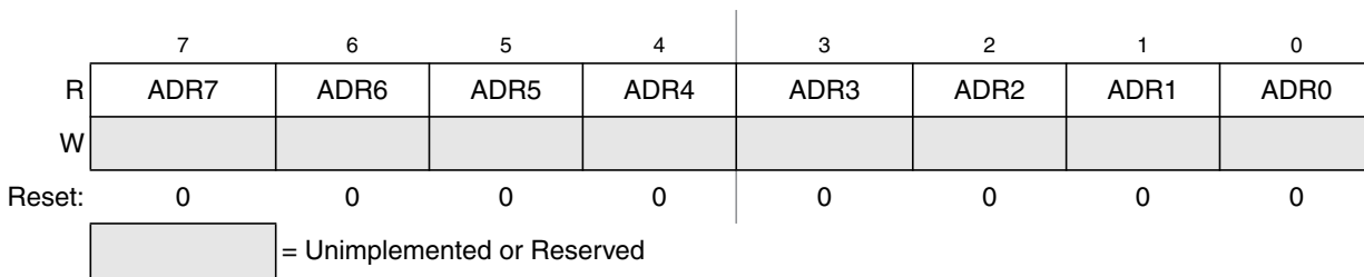
Figure 14-7. Data Result Low Register (ADC1RL)
