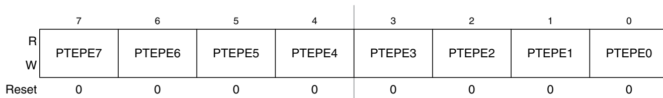
Figure 6-31. Internal Pullup Enable for Port E (PTEPE)
