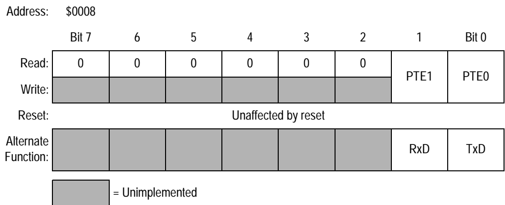
Figure 16-17. Port E Data Register (PTE)
