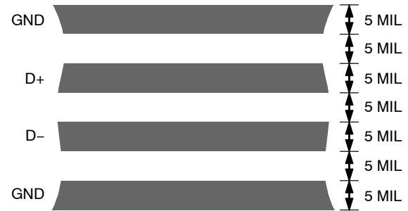
Figure 12. Typical Assignment of Signal Tracks
