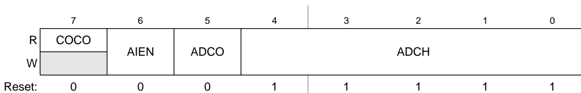
Figure 10-3. Status and Control Register (ADCSC1)
