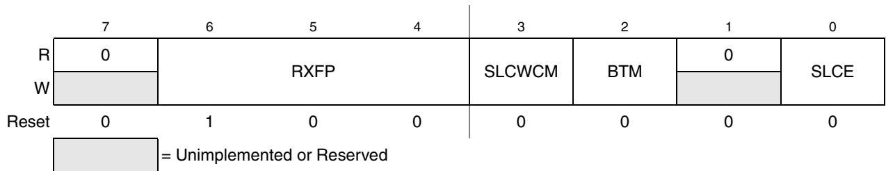
Figure 12-5. SLIC Control Register 2 (SLCC2)
