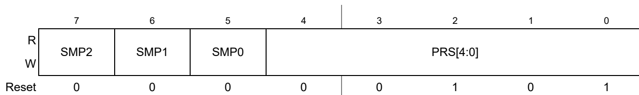
Figure 13-7. ATD Control Register 4 (ATDCTL4)
