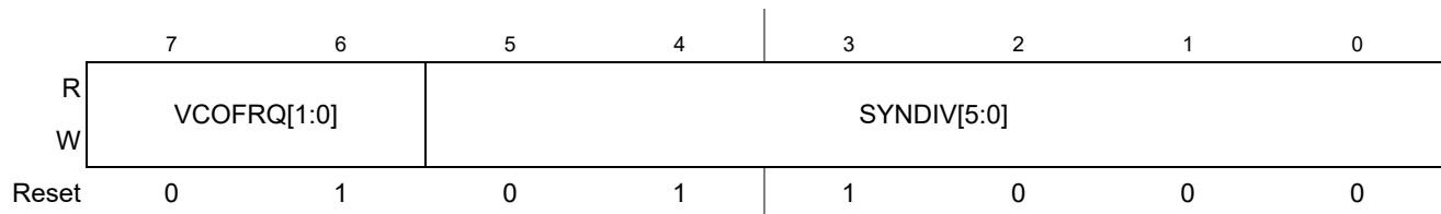
Figure 10-4. S12CPMU Synthesizer Register (CPMUSYNR)
