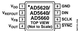
Figure 4. MSOP Pin Configuration
