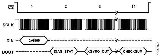
Figure 43. Burst Read Sequence with BURST_SEL = 0
