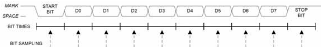
Figure 18.4. 8-Bit UART Timing Diagram
