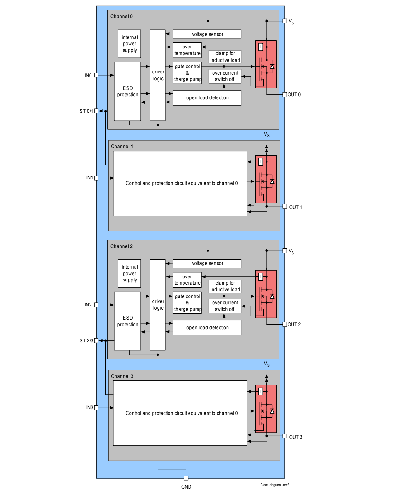
Figure 1 Block diagram for the BTS4130QGA
