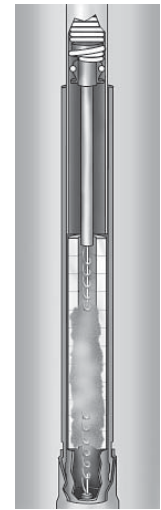
Vapor quenches arc at first current zero
