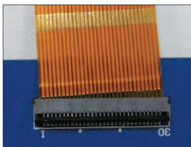
✗ Skewed FPC Insertion
