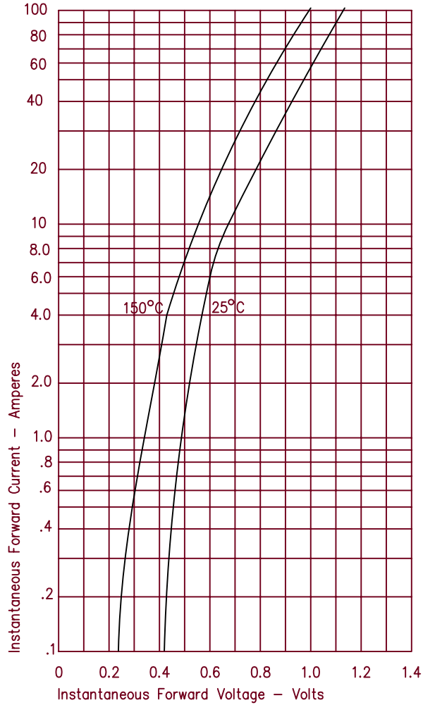
Figure 1 Typical Forward Characteristics
