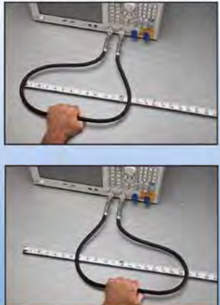
Cable is pulled off center 10" in both directions A brand new cable can have a break-in period of several hundred flexes
