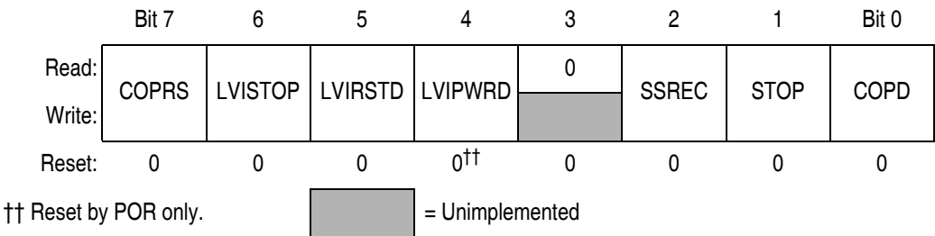
Figure 5-2. Configuration Register 1 (CONFIG1)
