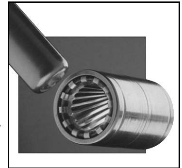
The RADSOK design - socket cylinder within female contact has twisted hyperbolic grid. Provides higher amperage capabilities with low insertion force and low temperature rise.
