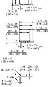
Lead coplanarity .102mm (.004 inch) max. at mounting surface.
