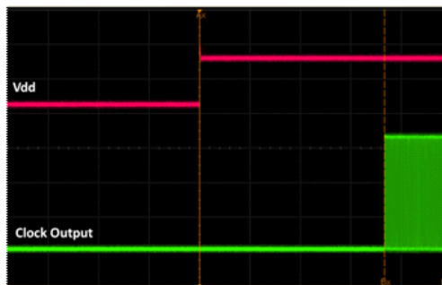
Figure 16. Startup Waveform vs. Vdd
