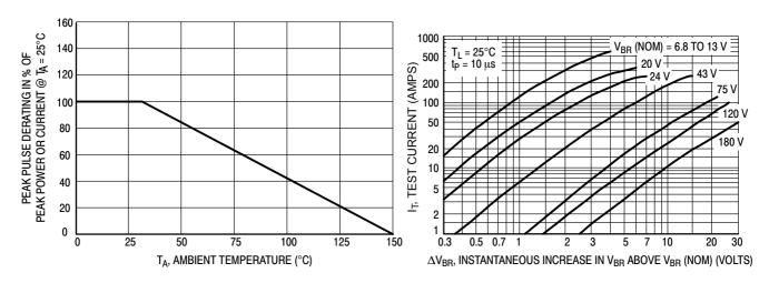
Figure 3. Pulse Derating Curve
