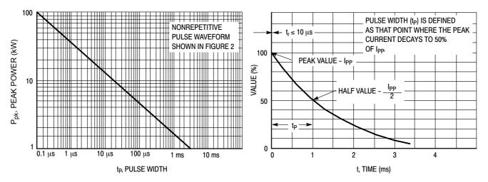
Figure 1. Pulse Rating Curve
