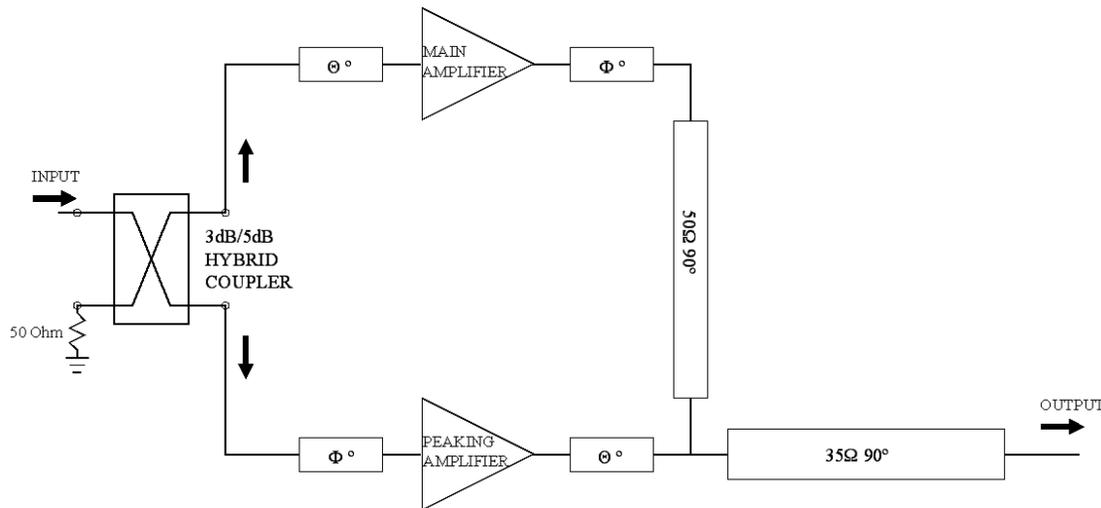
Hybrid coupler can be used in Doherty power amplifier to split the input power into the desired power ratio and phase delay. In above symmetrical Doherty power amplifier (main and peaking amplifier delivers equal amount output power at max drive condition), 3dB hybrid splits the input power into 1:1 ratio with 90 degree phase difference.
