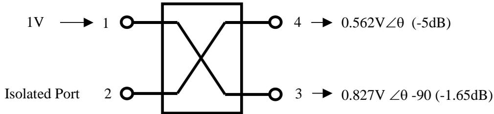
The primary application for 5dB couplers is in serial splitting and combining networks. These networks are often employed when the combining of 3 amplifiers is required. Unlike corporate networks, serial networks are not limited to binary divisions (corporate networks are limited to  $2^n$  number of splits, where  $n$  is an integer). Serial networks can be designed with [3, 4, 5, .....,  $n$ ] splits, but have a practical limitation of about 8 splits.
