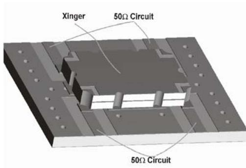
**Figure 3: Component Placement**
