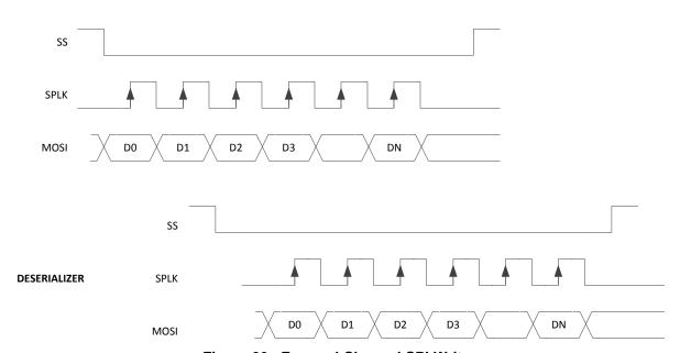
Figure 20. Forward Channel SPI Write
