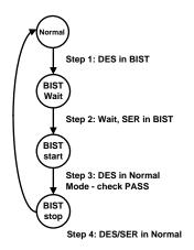
Figure 26. BIST Mode Flow Diagram
