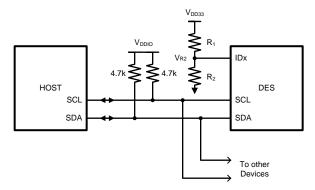
Figure 33. Serial Control Bus Connection
