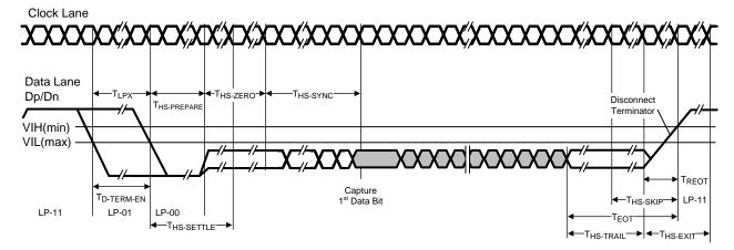
Figure 11. High Speed Data Transmission Burst
