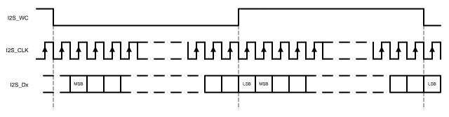
Figure 25. I2S Frame Timing Diagram
