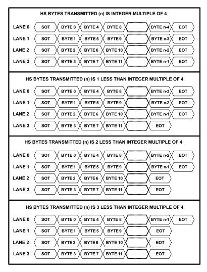
Figure 14. 4 MIPI Data Lane Configuration
