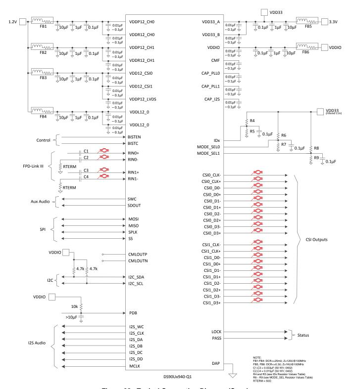
Figure 38. Typical Connection Diagram (Coax)
