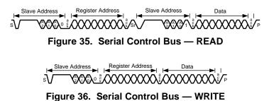
The I2C Master located at the Deserializer must support I2C clock stretching. For more information on I2C interface requirements and throughput considerations, please refer to TI Application Note SNLA131.
