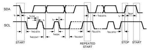
Figure 8. Serial Control Bus Timing Diagram
