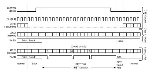
Figure 27. BIST Waveforms
