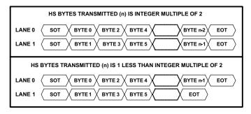
Figure 15. 2 MIPI Data Lane Configuration
