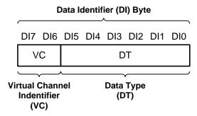
Figure 32. CSI-2 Data Identifier Structure
