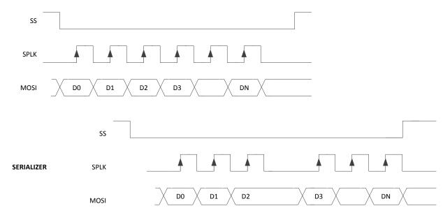
Figure 22. Reverse Channel SPI Write
