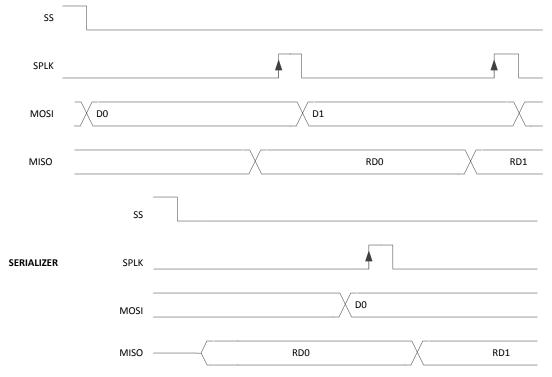
Figure 23. Reverse Channel SPI Read
