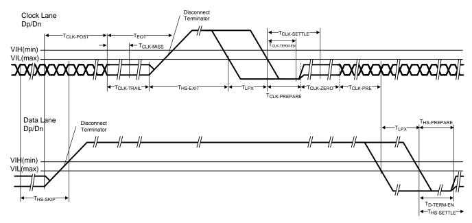
Figure 12. Switching the Clock Lane between Clock Transmission and Low-Power Mode
