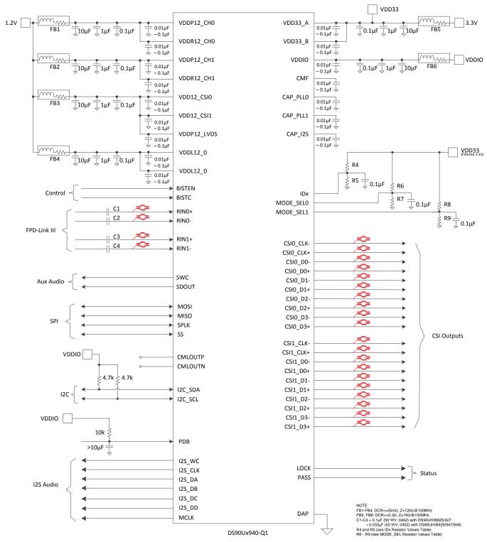
Figure 37. Typical Connection Diagram (STP)
