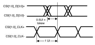
Figure 10. Clock and Data Timing in HS Transmission
