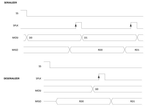
Figure 21. Forward Channel SPI Read
